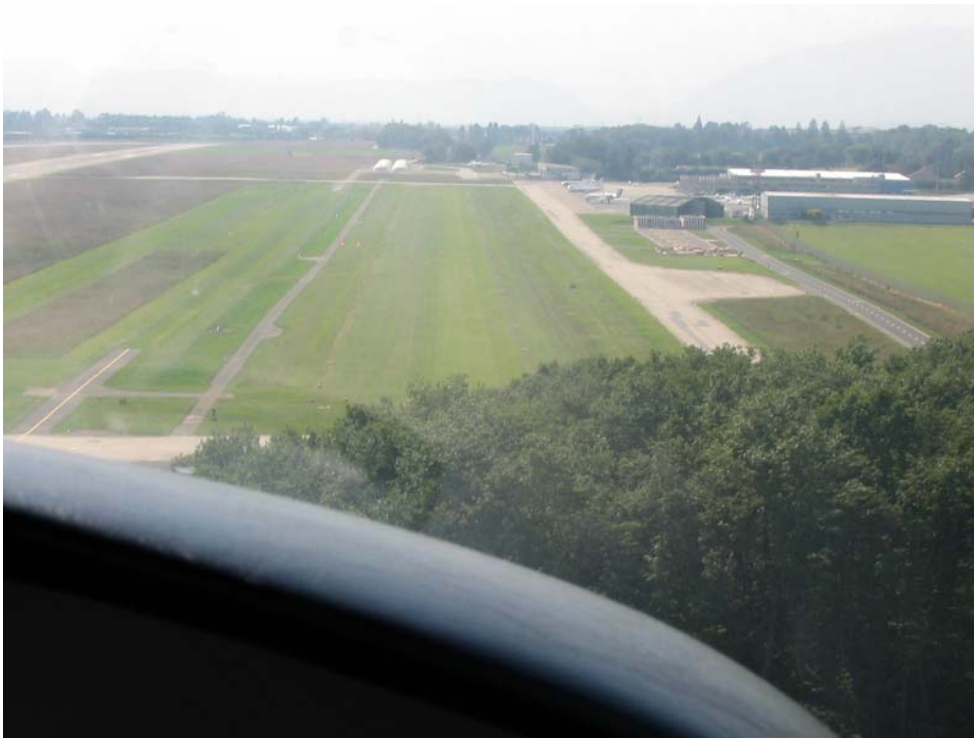
Figure 2-8. Approach to grass RWY 23, over the same trees as depicted in Figure 2-3. Close inspection of the illustration reveals that the APAPI lights to the left of grass RWY 23 are both red, indicating that the aircraft is below the nominal approach path.
